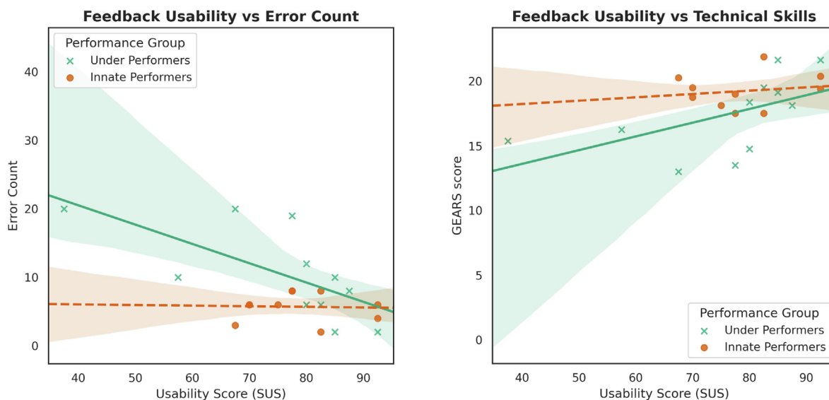
Fig. 3 – Empirical correlation of the System Usability Scale (SUS) score with the error count and technical skills score (GEARS) for underperformers and innate performers. The difference in slope shows that the feedback was more important in helping underperformers than innate performers. GEARS = Global Evaluative Assessment of Robotic Surgery.
