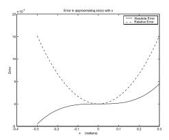
Although the absolute error is relatively flat around x=0, the relative error grows more quickly. The relative error reflects the fact that the absolute value of  $\sin(x)$  is small near x=0.
