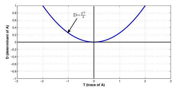
This graph is an example of a parameter plane. As the matrix A changes it has different values of T and D and the linear system  $\frac{d\vec{x}}{dt} = A\vec{x}$  corresponding to that matrix will be located at a different location in (T, D)-space.
